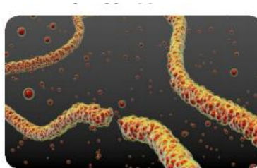
Figure 2: Illustration of nanocapillary bridged filaments assembled into 2D gel-like network. The network upon mechanical damage can be repaired by external magnetic field, highlighting the self-healing properties of filaments.
